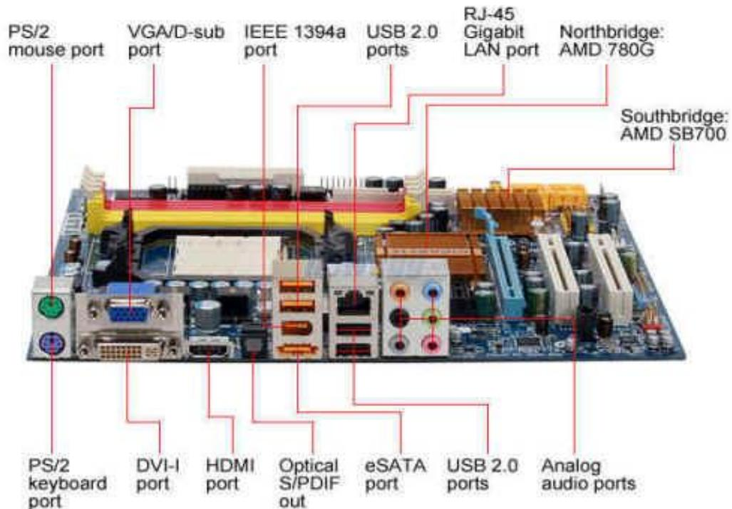
**9. eSATA port (External Serial Advanced Technology Attachment):** It is an external interface for SATA technologies. It competes with FireWire 400 and universal serial bus (USB) 2.0 to provide fast data transfer speeds for external storage devices.
