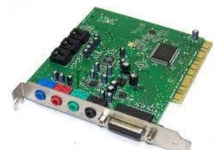
In order to play and record sounds, a card needs to connect to at least a set of speakers and a microphone. Sound cards have two miniature audio jacks for a microphone and a speaker, also line in to record from a stereo or tape recorder, line out to output sound and a female 15-pin DB socket to attach an electronic musical instrument or a joystick to your PC.
